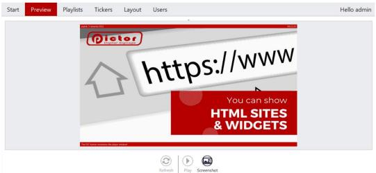
In the *Preview* menu, you can see the player's screen. You see exactly what is being shown on the screen at the time. The delay is up to a maximum of 2 seconds. In addition, at the top of the screen you can expand the window and see the content data displayed on each region. The preview works in the following modes:
